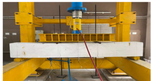
Fig. 7 Fully Steel Reinforced beam Testing
