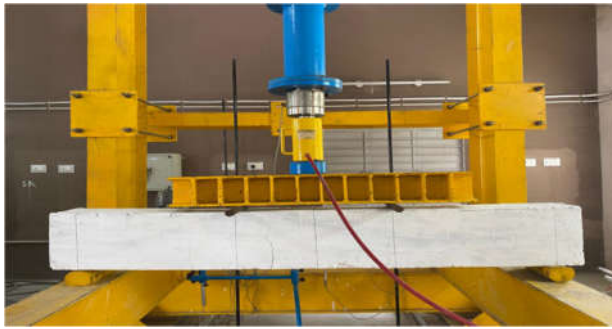
Fig. 8 Fully GFRP Reinforced beam Testing
