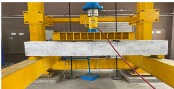
Fig. 9 Hybrid Reinforced beam Testing
