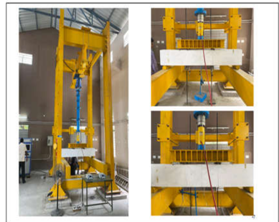
Fig. 6 Loading Frame beam Testing
