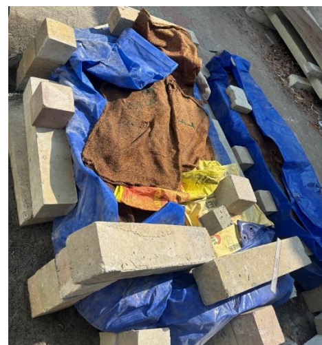
Fig.7 Curing Of Column Specimens.
