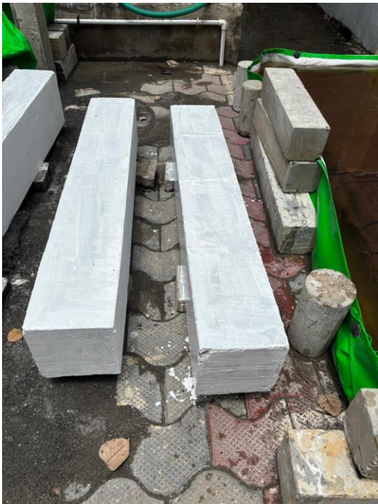
Fig.8 Preparation Of Column Surface For Testing Using White Emulsion
