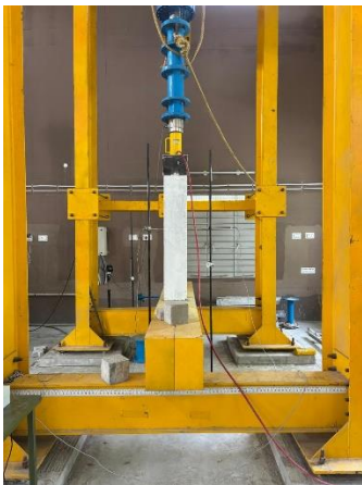
Fig.11 Columns Test Setup
