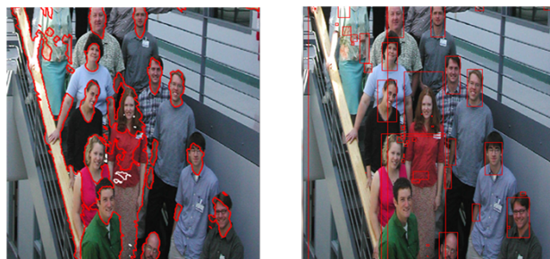
(a) Result Skin-Color Regions obtained after Merge Skin-Color Regions (b) Skin-Color Regions obtained after Labeling and Non-Face Region Rejection
