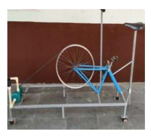
Make a pedal operated centrifugal pump, where the pump will work on the principle of pedaling .The other important components used to make this pedal operated centrifugal pump is centrifugal pump, cycle rim, nuts and bolts, v-belt, square shape rods, chain pedal .
