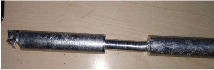
Fig. 5 UTS test specimen of HMMC
