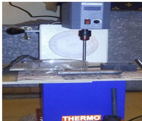
Fig. 1 Top opening furnace with stirrer
