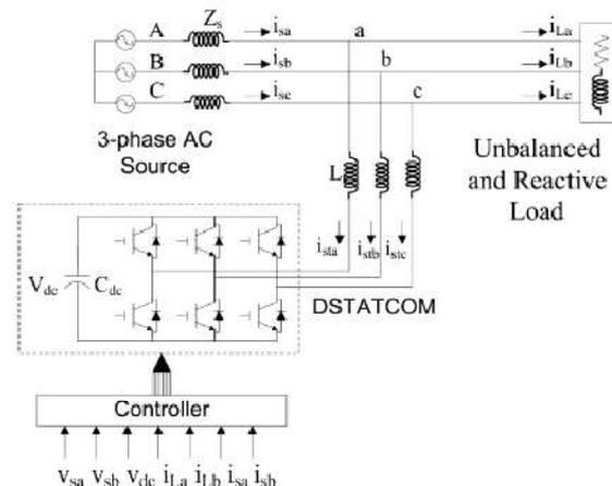
**Fig.2. Basic Circuit Diagram of the DSTATCOM System.**
