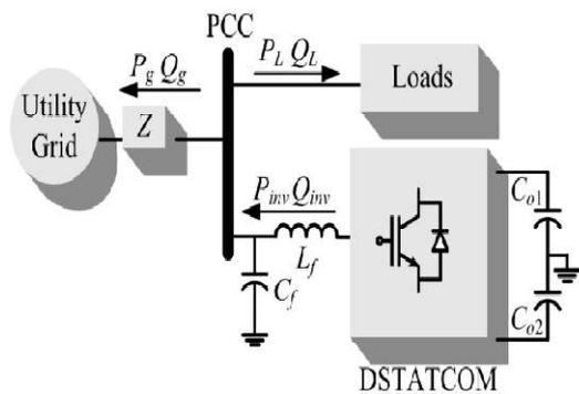
**Fig. 1. Low voltage distribution grid under analysis with the voltage regulator**
