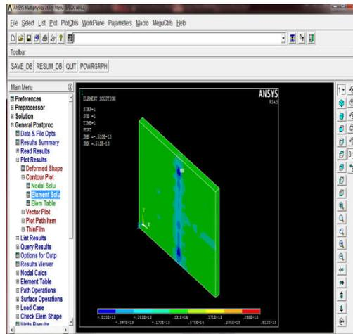
Fig.4.1 Heat flow in masonry wall
