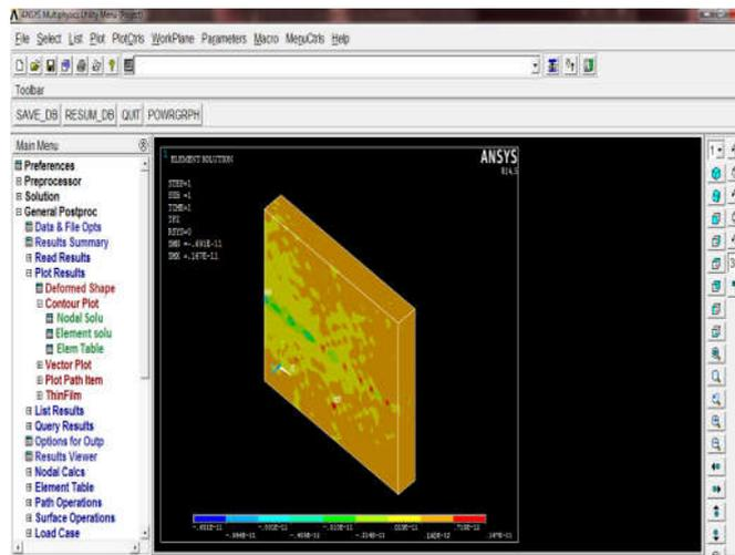
Fig.4.4 Heat flux in PCM wall
