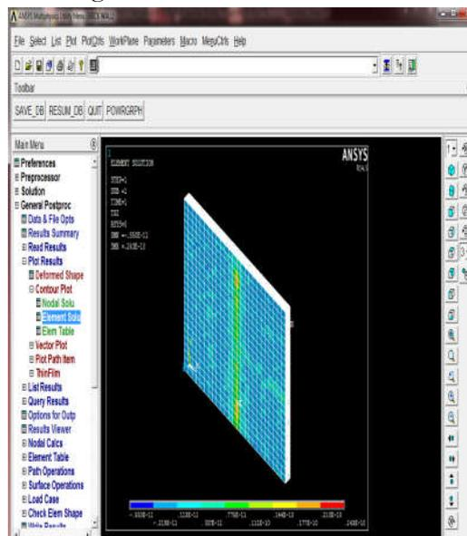
Fig.4.5 Thermal gradient in masonry wall
