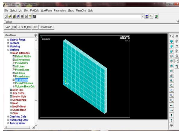
Fig.3.4 Meshing of ordinary wall
