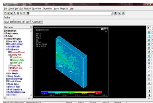
Fig.4.6 Thermal gradient in pcm wall
