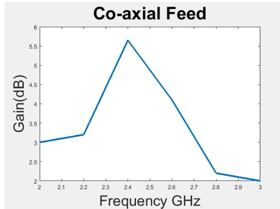
(b) Frequency versus Gain of coaxial Feed
