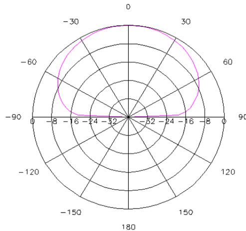
Fig. 17 2D E-plane Radiation pattern of Inset-fed ETMSA
