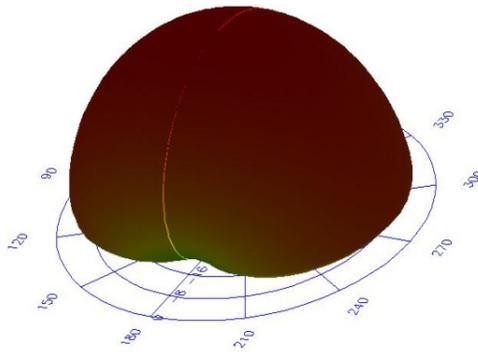
Fig. 4 (a) 3D - E-Plane Radiation Pattern of Line fed ETMSA
