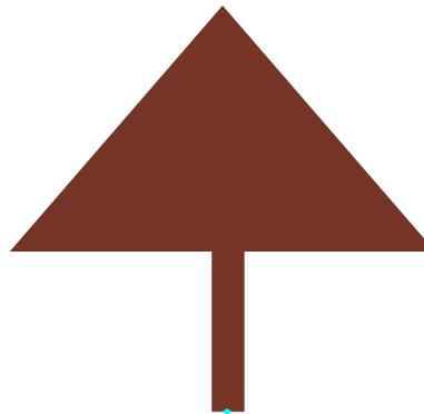
Fig. 2 Layout of Line fed ETMSA
