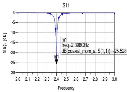
Fig. 12 (a)  $S_{11}$  of Coaxial fed ETMSA
