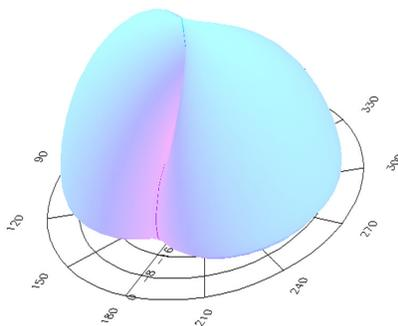
Fig. 13 (a) 3D- E-Plane Radiation pattern of coaxial fed ETMSA
