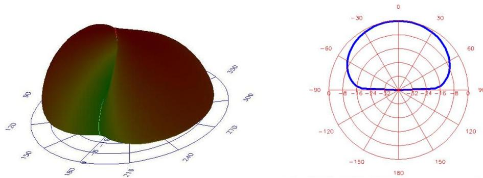
Fig. 9 (a) 3D – E-Plane Radiation Pattern of Inset fed ETMSA (b) 2D- E-Plane Radiation pattern of Inset fed ETMSA
