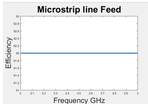
Fig. 5 Frequency versus efficiency of Line fed ETMSA
