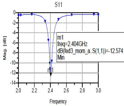
Fig.3 (a) S<sub>11</sub> of line fed ETMSA
