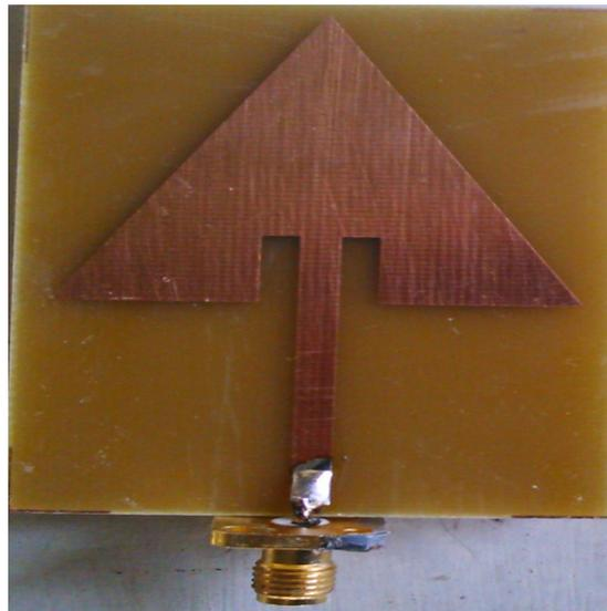
Fig. 15 Fabricated Prototype of Inset-fed ETMSA
