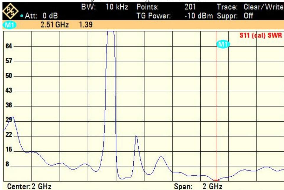
Fig. 16 Measured VSWR for Inset Microstrip Antenna
