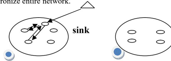
Fig.3.2 Sink sends message to cluster head and for other nodes
