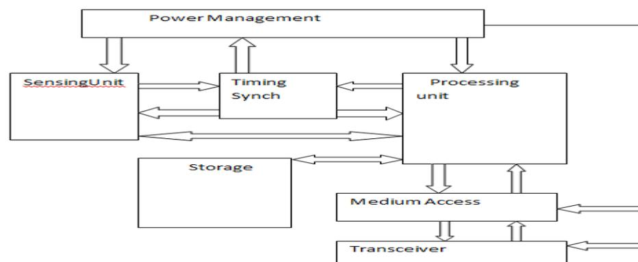
Figure 1.1: Schematic diagram of a sensornode
