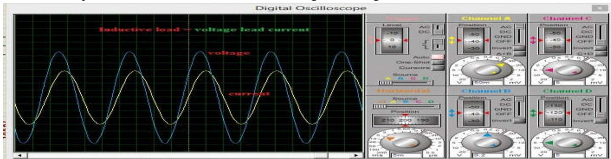
GRAPH 3.1.3 OSCILLOSCOPE WHEN INDUCTIVE LOAD IS ON
