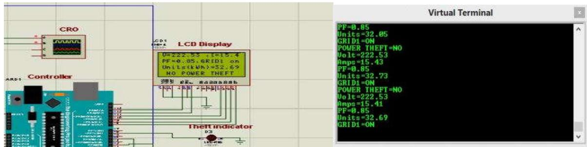
Figure 3.1.4 a) DISPLAY READING AT INDUCTIVE LOAD IS ON b) VIRTUAL TERMINAL AT INDUCTIVE LOAD
