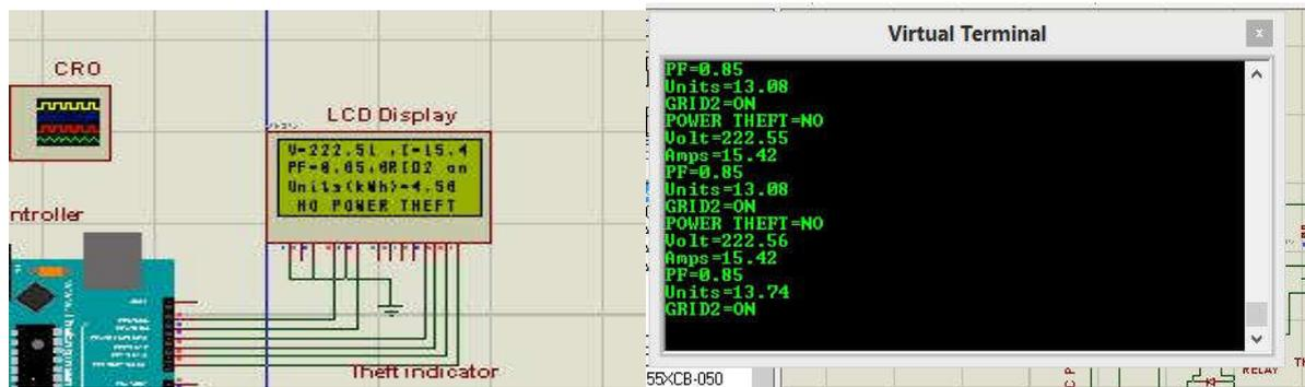
Figure 3.1.9 a) LCD DISPLAY when Grid 2 is ON b) VIRTUAL TERMINAL READINGS when Grid 2 is ON
