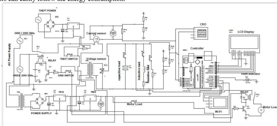
FIGURE 2.2(a): CIRCUIT OF IOT BASED SMART GRID
