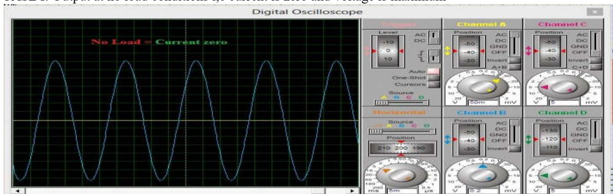
GRAPH 3.1.1 oscilloscope value at no load
