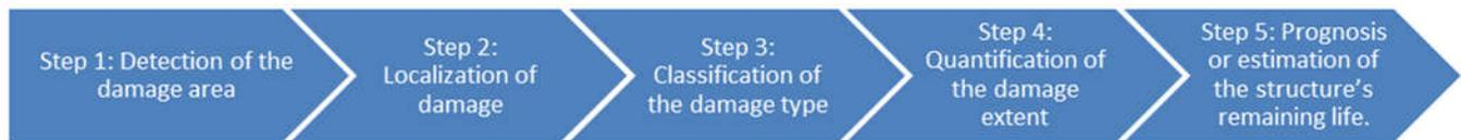
Fig. 1 Basic steps involved in Structural Health Monitoring
