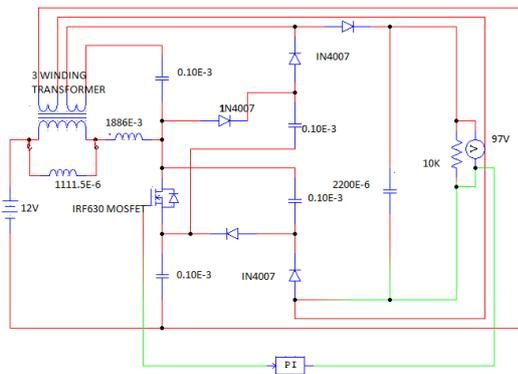
Fig.1. Circuit configuration of the proposed converter.
