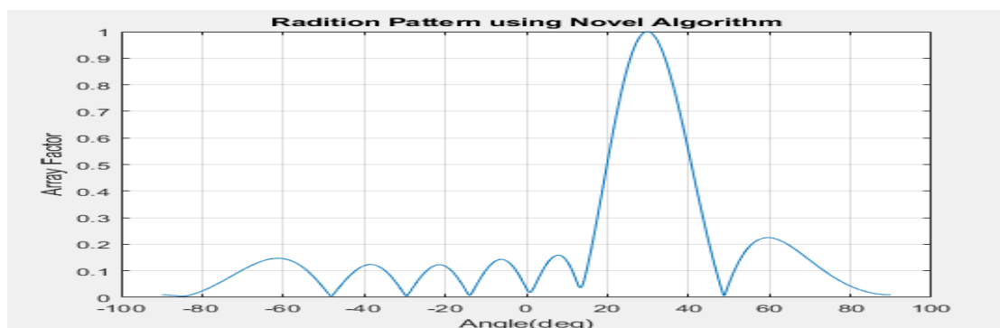
Figure 4: Radiation Pattern for Feedback Loop VSSLMS Algorithm in Beam Plot Format
