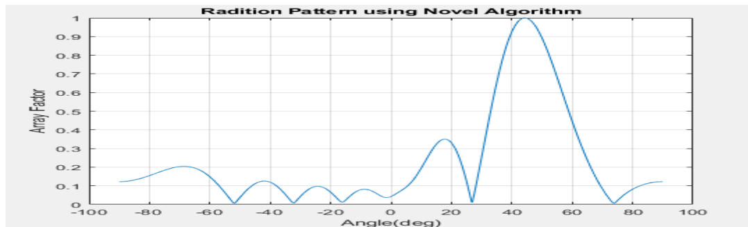
Figure 10: Radiation Pattern of VSSLMS Feedback Algorithm in Beam Plot Format for More number of Antenna Elements and Multiple Interference
