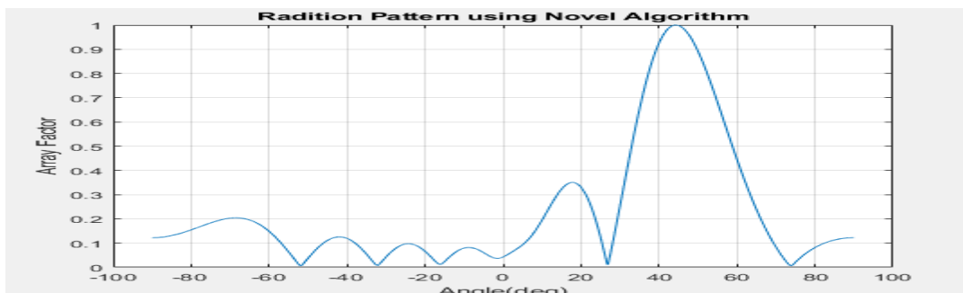
Figure 6: Radiation Pattern of VSSLMS Feedback Algorithm in Beam Plot Format for Less number of Antenna Elements and Multiple Interference
