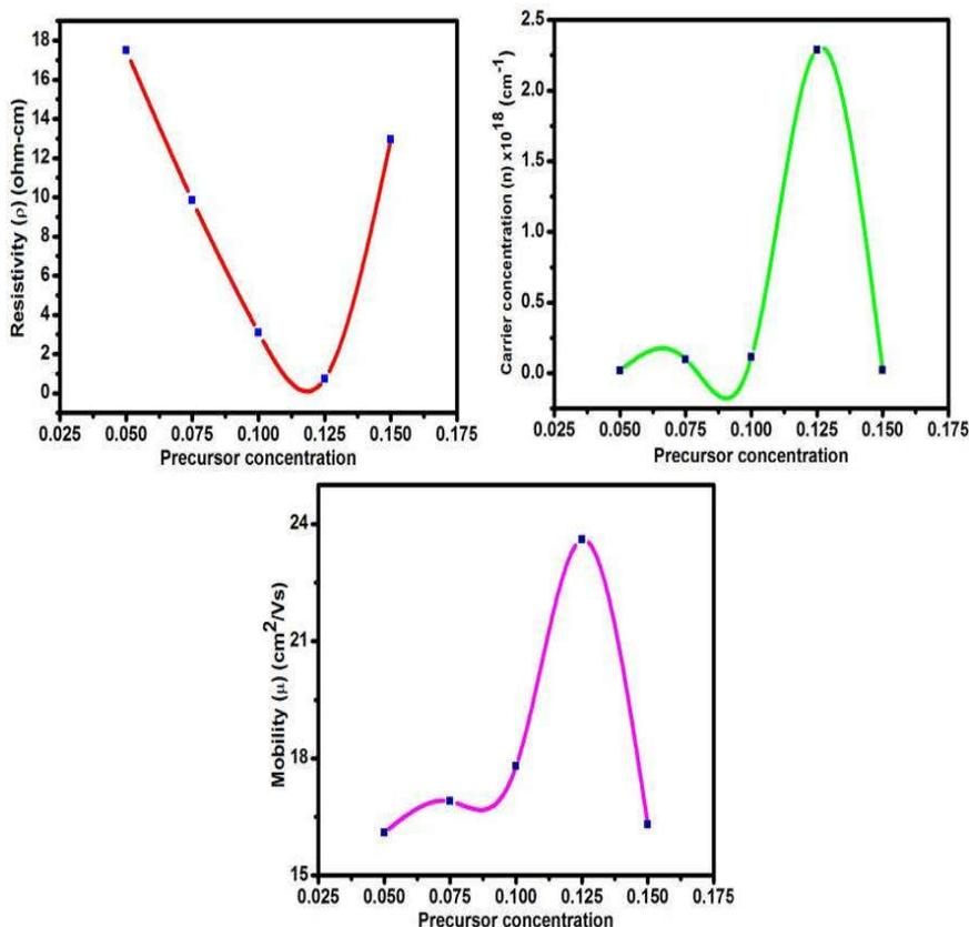
Fig.8 Variation of resistivity, carrier concentration and mobility of SnS thin films of different precursor concentration
