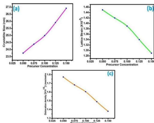
Fig. 3 The variation of structural parameters with different precursor concentration of SnS thin films
