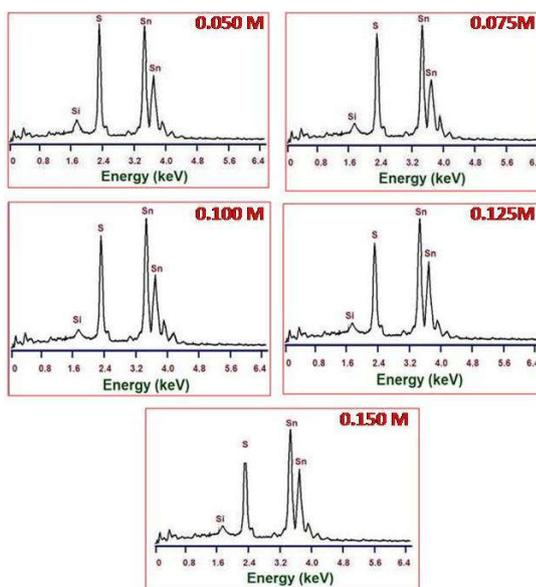
Fig.5 Energy dispersive X-ray (EDX) pictures of SnS thin film for different precursor concentration
