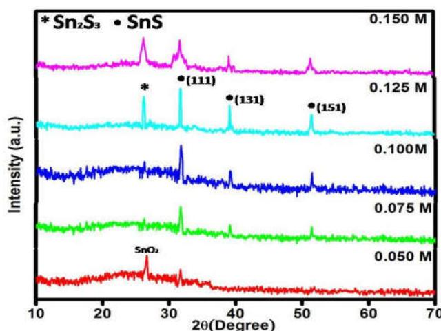
Fig.1 X-ray diffraction pattern of nebulized spray deposited SnS thin films at Different precursor concentration
