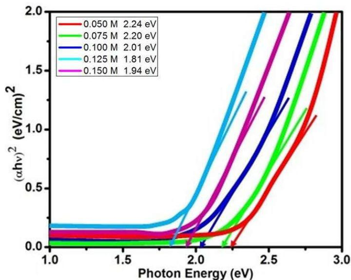
Fig.7 Plot of  $(\alpha h\nu)^2$  versus Photon Energy for nebulized spray deposited SnS thin films for different precursor concentration
