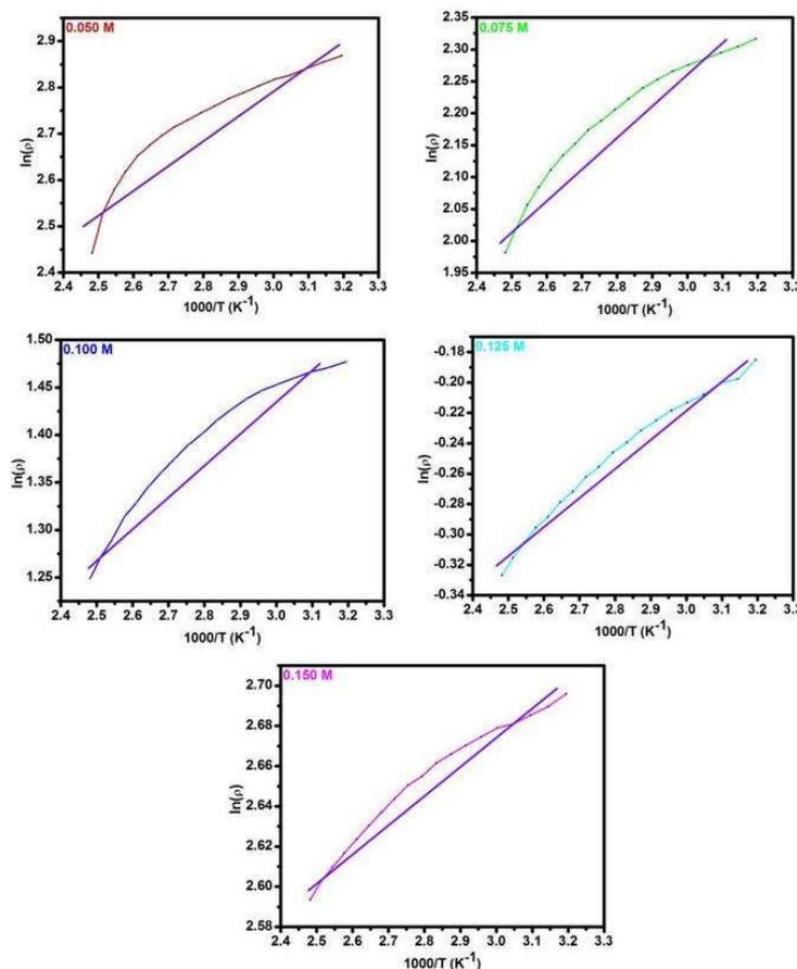
Fig. 9 Arrhenius Plot for SnS thin films for different precursor concentration
