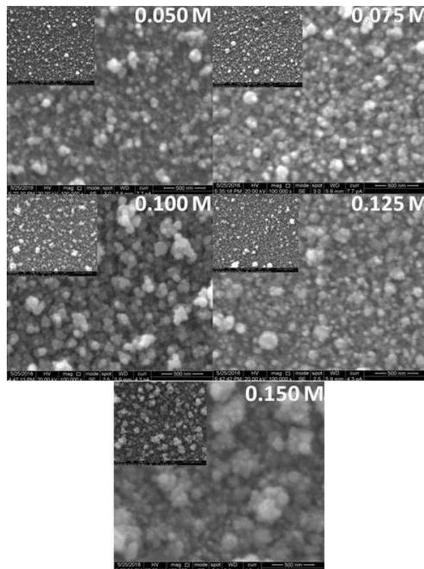
Fig .4 Scanning electron microscope (SEM) images of SnS thin films for different precursor concentration
