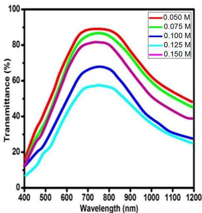
Fig. 6 Wavelength versus transmittance spectra of nebulized spray deposited SnS thin films
