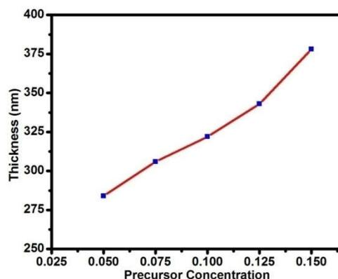
Fig.2 Variation of thickness of SnS thin films at different precursor concentration
