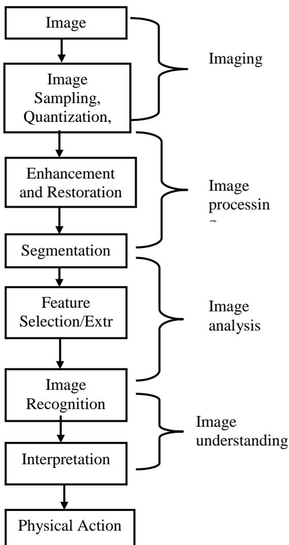
Fig. 1 Image processing block diagram
