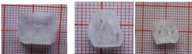
Figure1: photographs of grown crystals of pure LASS,  $\text{Mn}^{2+}$  doped,  $\text{Mg}^{2+}$  doped LASS respectively
