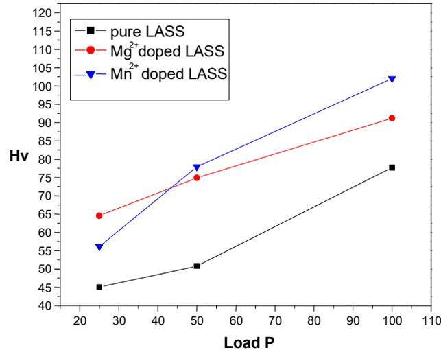
Fig. 6. Hardness behavior of pure and doped LASS
