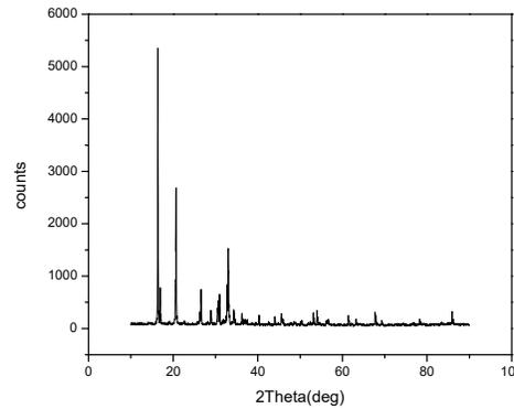
Figure 4: powder XRD pattern of  $Mg^{2+}$  doped LASS
