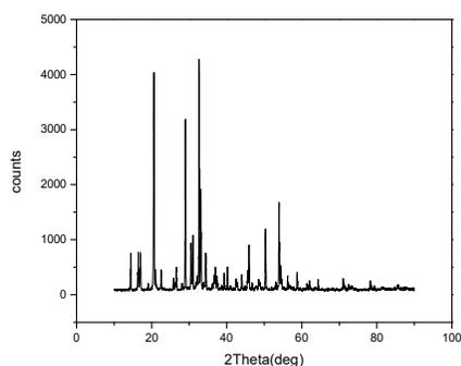
Figure 2: powder XRD pattern of pure LASS
