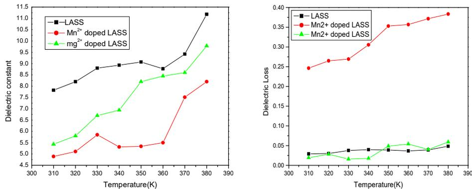
Fig.8: Dielectric constant Vs temperature for 10<sup>3</sup> KHz Fig.9: Dielectric Loss Vs temperature for 10<sup>3</sup> K Hz
