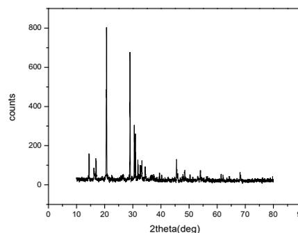
Figure 3: powder XRD pattern of  $\text{Mn}^{2+}$  doped LASS
