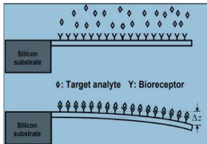
**Figure 1: Working of a Cantilever Array Biosensor**
