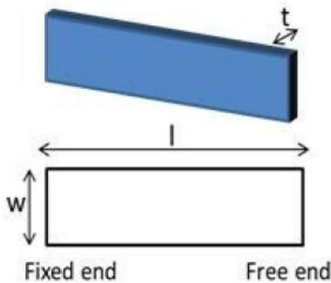
**Figure 2a: Design of Micro Cantilever Beam**
