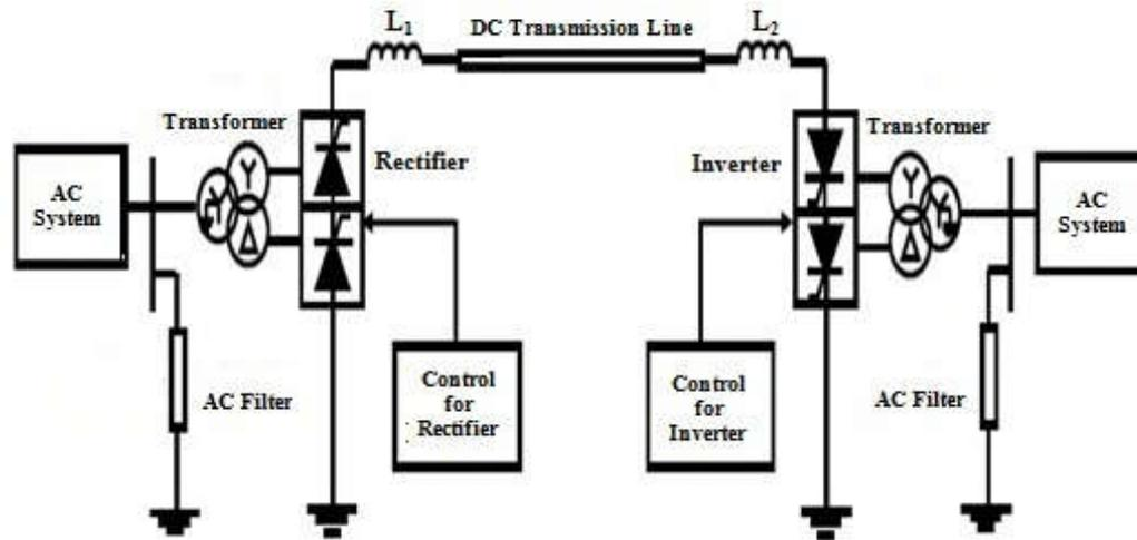
Figure 1: The monopolar HVDC transmission system model
