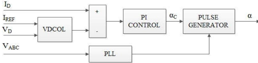
Figure 2: Logic diagram of the rectifier control system model.
