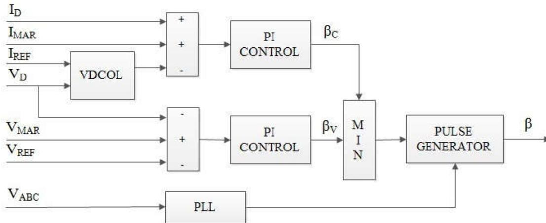
Figure 3: Logic diagram of the inverter control system model.
