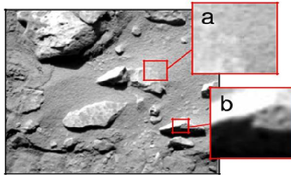
**Figure 1** Rocks diverse textures, variable morphologies, and directional illumination all complicate the segmentation problem. Local cues are insufficient: real borders are often weak (a), while the rocks themselves are non-uniform with false interior borders
