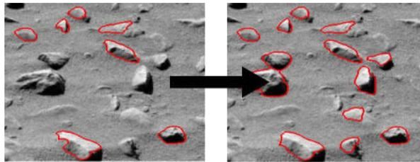
**Figure 4: The effect of the configuration search on rock segmentation results. The initial segmentation (left) loses rocks whose probabilities fall below the confidence threshold. The search process recovers their boundaries and improves their score (right).**
