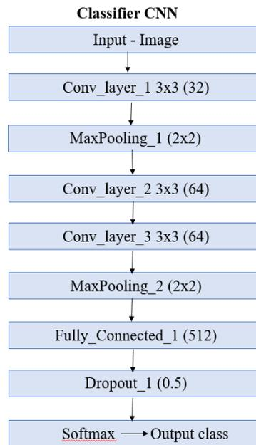
Fig 2: The proposed CNN Architecture for classification
