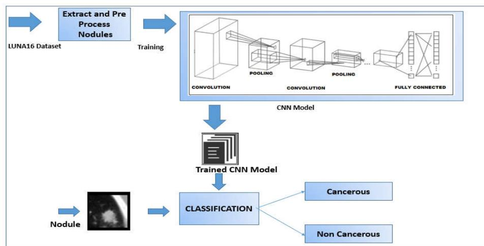
Fig 1: System Architecture of Lung cancer detection using Convolutional Neural Network
