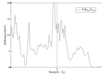
Figure 5: DOS of Fe<sub>0.5</sub>Co<sub>0.5</sub>Se
