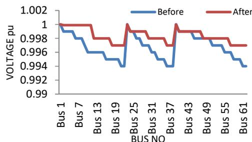
Fig. 11. Comparison of Bus voltages before and after reconfiguration 62 bus
