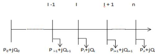
Fig. 1. Single line diagram of a distribution network
