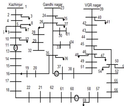
Fig.12.Single line diagrams of three substations with 62 buses (after reconfiguration)
