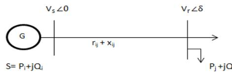
Fig: 2. Single line diagram of two bus system.
