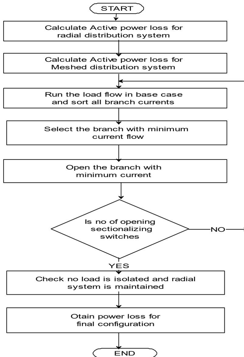
Fig.3. Flow chart of minimum current flow method.
