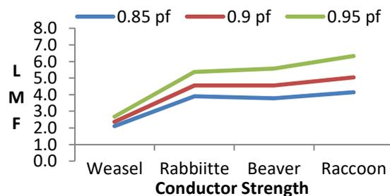
Fig. 6. Various conductors’ strength for different power factor
