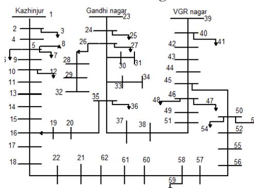
Fig. 8. Single line diagrams of three substations with 62 buses (before reconfiguration)
