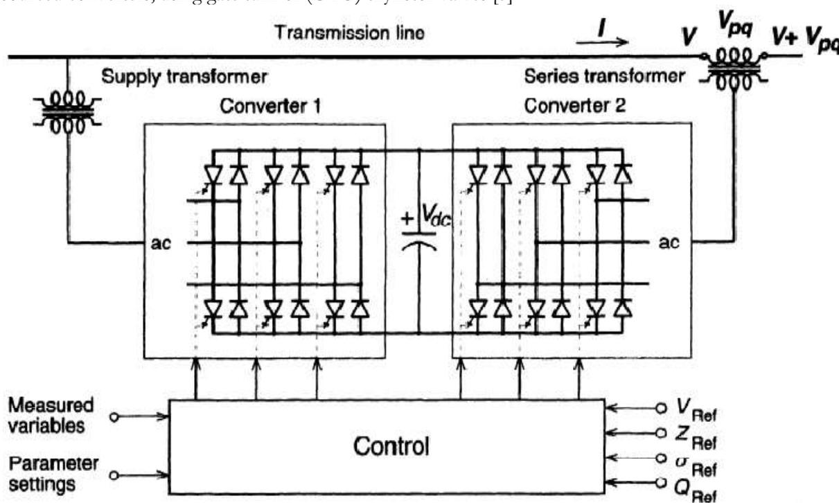
Figure 2. Unified power flow controller
