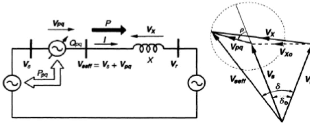
Figure 3. Conceptual representation of Unified Power flow Controller
