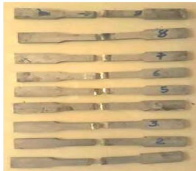
Fig. 8 Weldments after tensile testing
