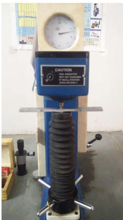
Fig. 4 Rockwell hardness tester available at CHARUSAT.
