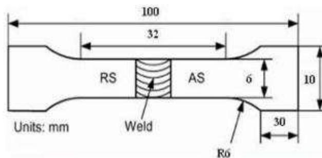
Fig. 5 Dimensions as per ASTM E8 standard for tensile testing.
