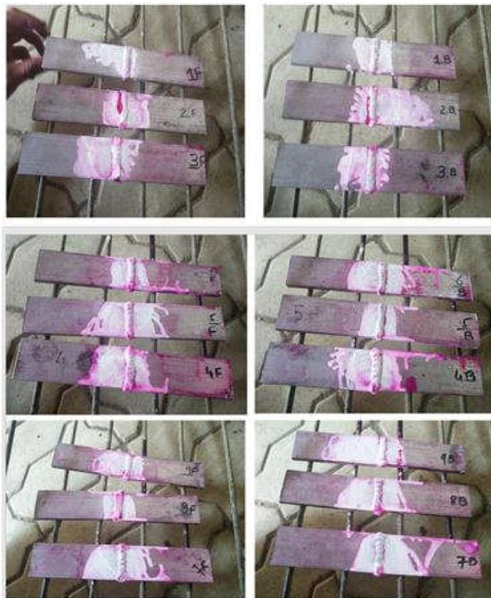
Fig. 3 Dye penetrate test done on prepared weldments of AA 6061
