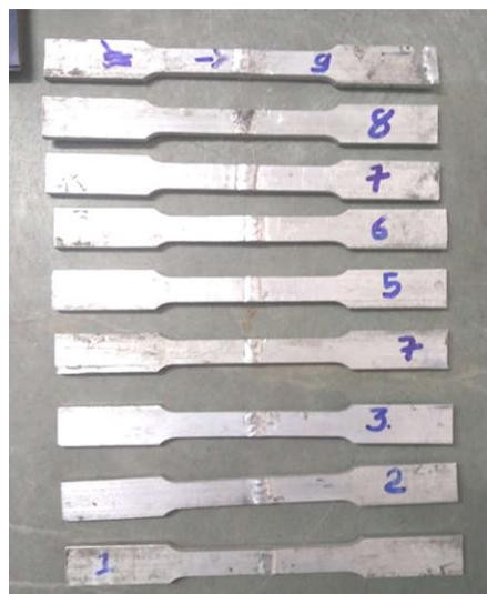
Fig. 6 Tensile specimens prepared for testing.
