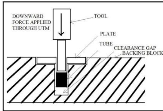
Fig.7.shear test setup
