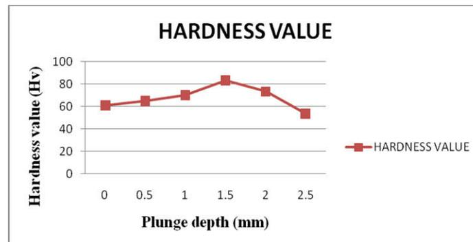
Fig.6. Plunge depth vs. Micro Hardness
