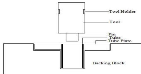
Fig.1. Schematic diagram of FWTPET
