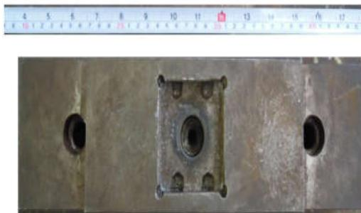
Fig. 3 Backing Block Used For FWTPET
