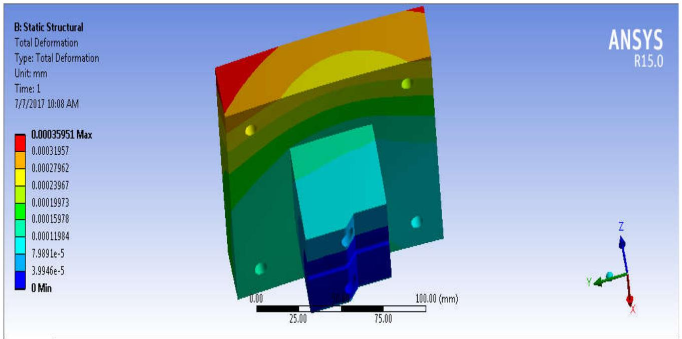
Fig.6 Total deformations of Top die for Wire bending operations
