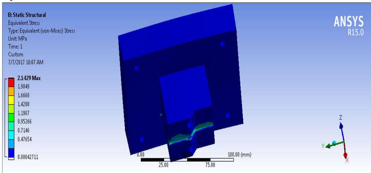
Fig.5 Equivalent stresses of Top die for Wire bending operations
