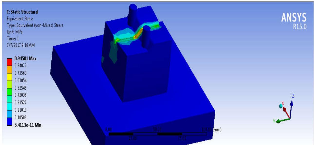
Fig.7 Equivalent stresses of Bottom die for Wire bending operations
