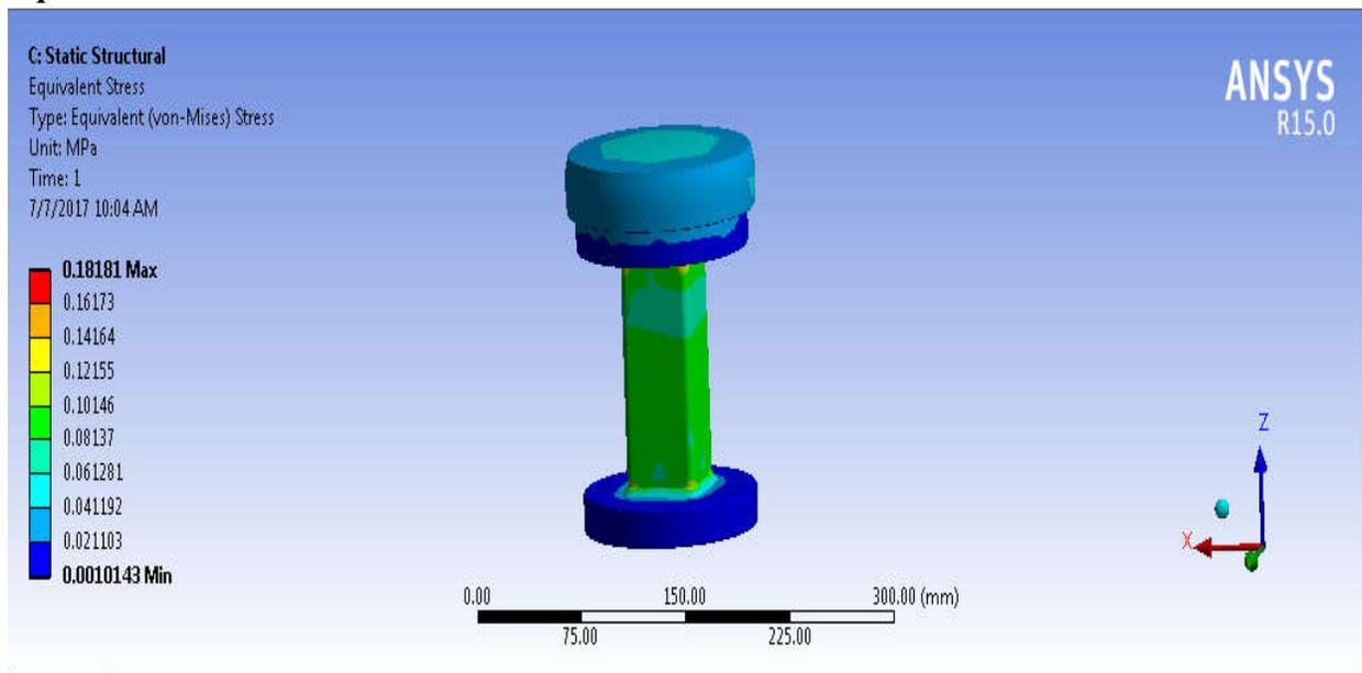
Fig 3 Equivalent stresses of Bottom die for ring sizing operations
