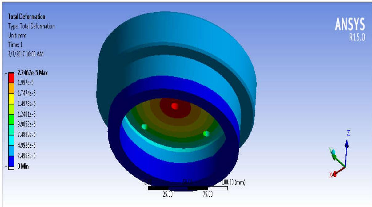
Fig.2 Total Deformation of top die for ring sizing operations
