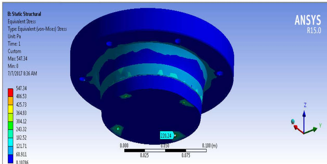
Fig.9 Equivalent Stress of Top die for Forming operations
