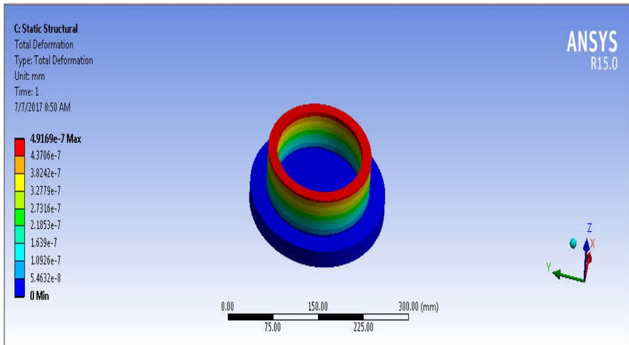
Fig.12 Total Deformation of Bottom die for Forming operations
