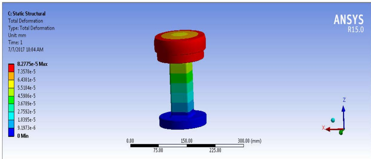
Fig 4 Total Deformation of Bottom die for ring sizing operations
