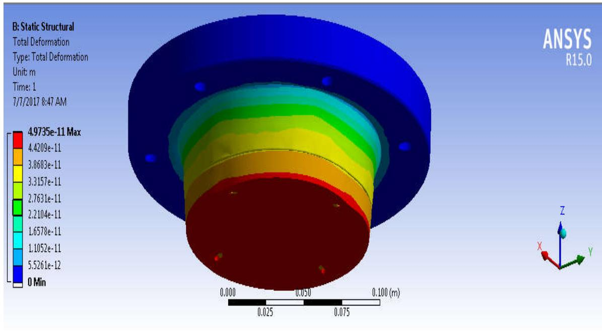
Fig.10 Total Deformation of Top die for Forming operations
