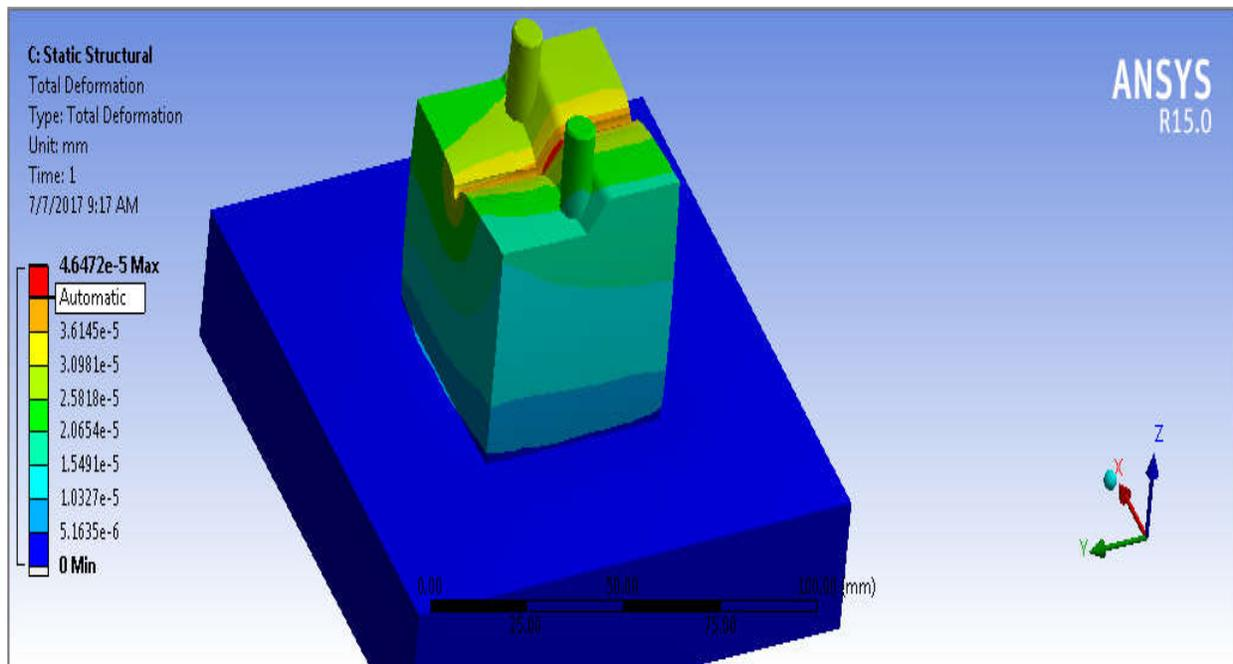
Fig.8 Total Deformation of Bottom die for Wire bending operations
