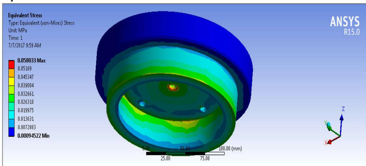
Fig. 1 Equivalent stresses of top die for ring sizing operations
