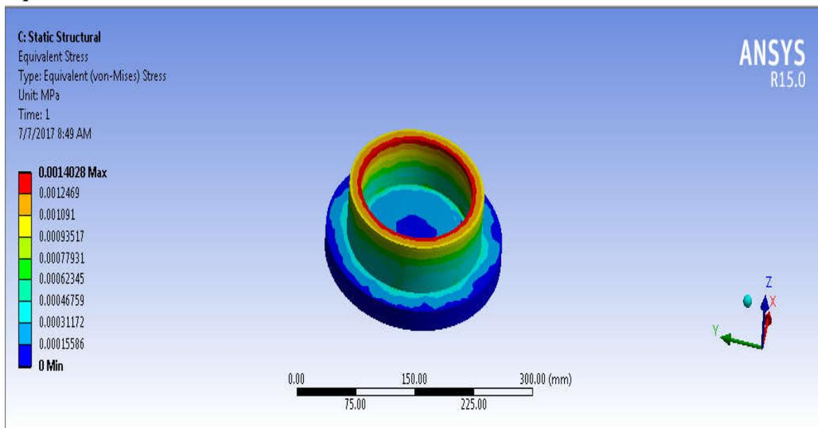
Fig.11 Equivalent Stress of Bottom die for Forming operations
