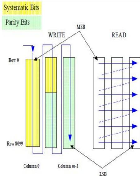
Fig 2: Row-column interleaver
