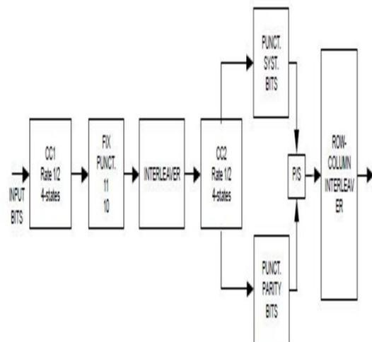
Fig.1: Block diagram of SCCC scheme
