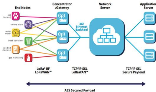
Fig. 1. Architecture of LoRaWAN Network
