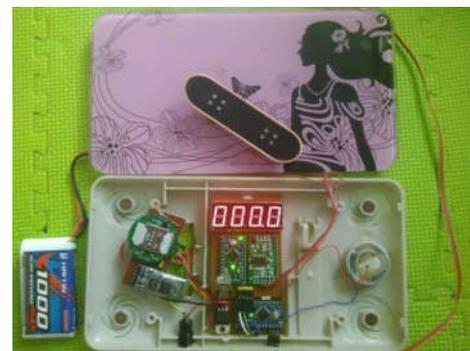
Fig. 7 Prototype of smart waste-bin.
