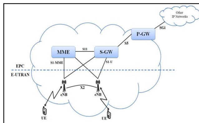
**Figure 1:** LTE-Advanced Network Architecture [2]
