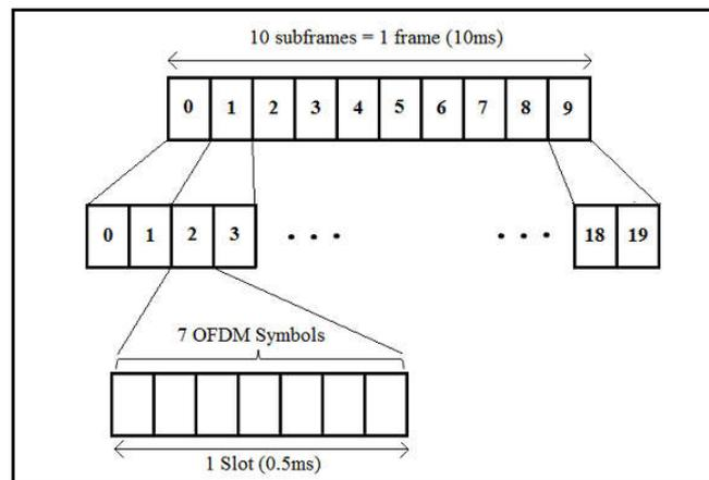
Figure 2: LTE Downlink Frame Structure [3]
