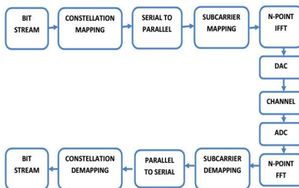
Figure 3: OFDM System Model
