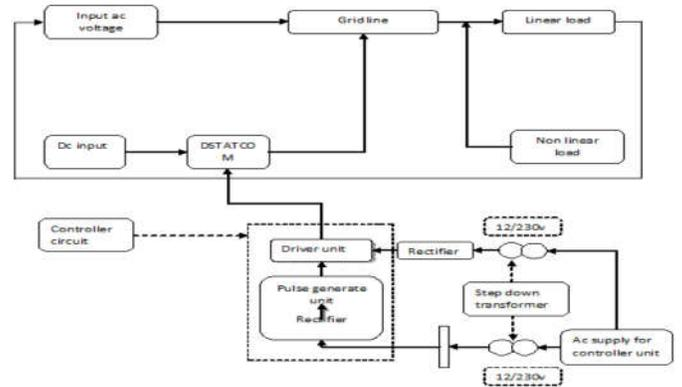
Fig.2 proposed block diagram
