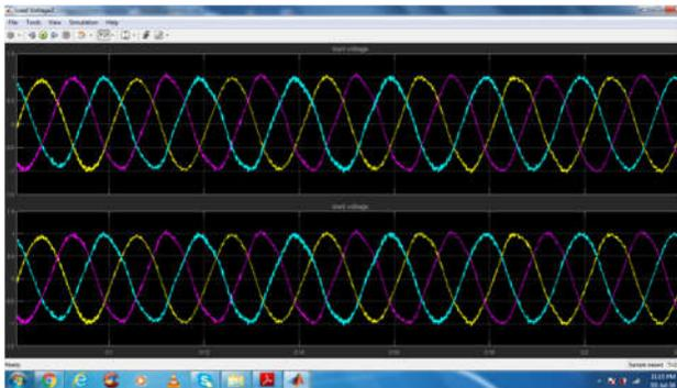
Fig 6 PCC voltages with and with out compensation for linear loads
