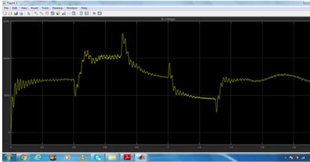
Fig 5 DC bus voltages during the DSTATCOM initialization
