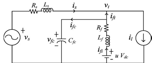
Fig.3 single phase equivalent circuit of STATCOM
