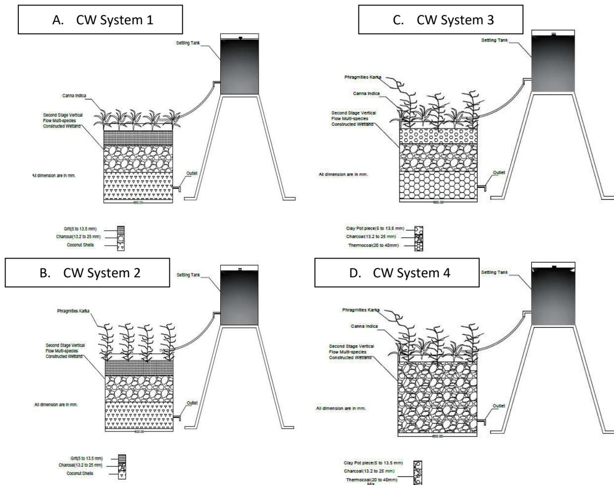
Fig. 1: Schematic Sketch of laboratory scale experimental set-up
