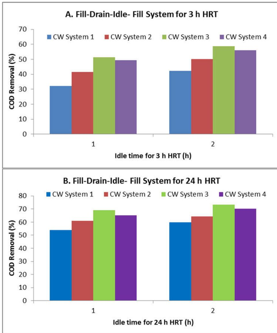
Fig. 4: Effect of idle time on COD removal for A) 3 h HRT and B) 24 h HRT in FDIF system
