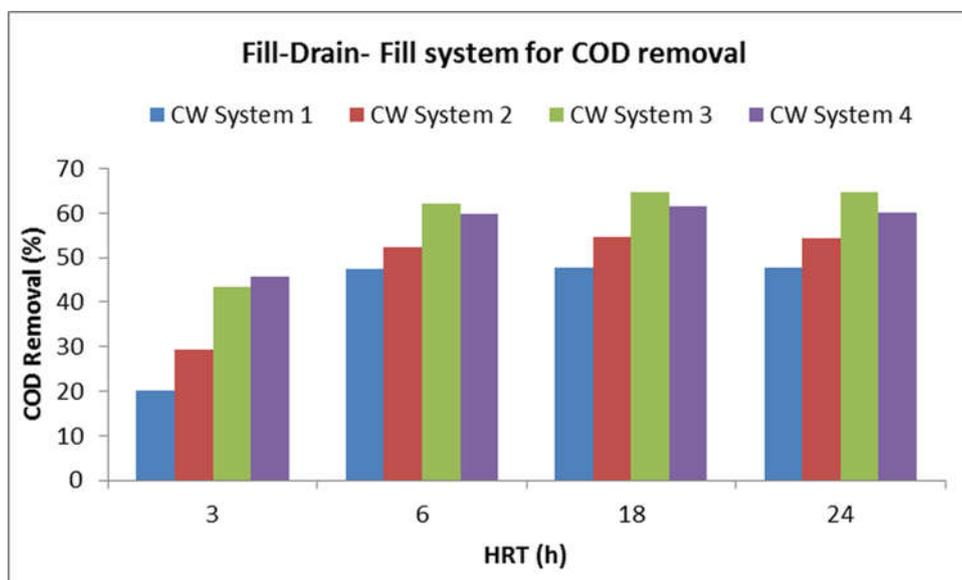
Fig. 2: Effect of HRT in FDF mode of system operation on COD removal
