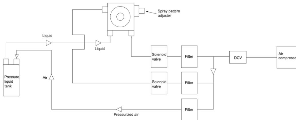
Fig 4:- Block diagram for coolant spray working.
