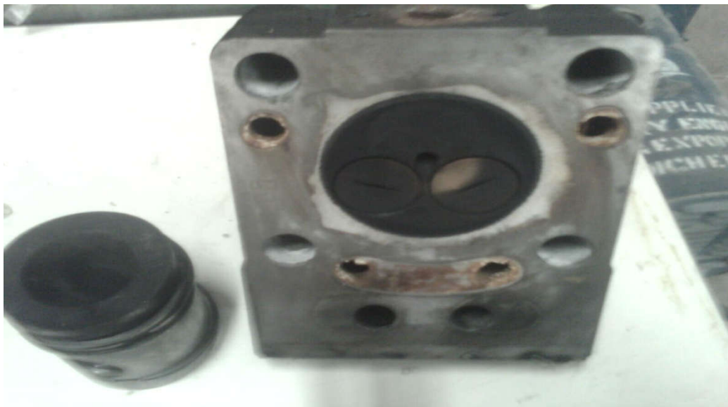
Figure 3: Zirconium Oxide coated piston and head
