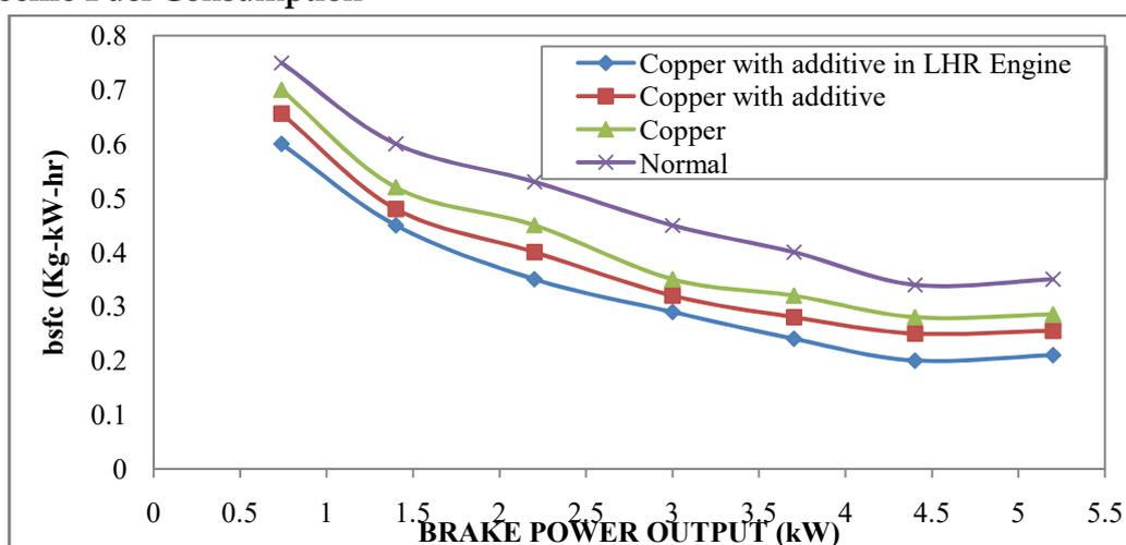
Figure 5: Variation of Brake Specific Fuel Consumption with power output for Iso-amyle Nitrate Fuel additives in Copper GHSI -LHR Engine
