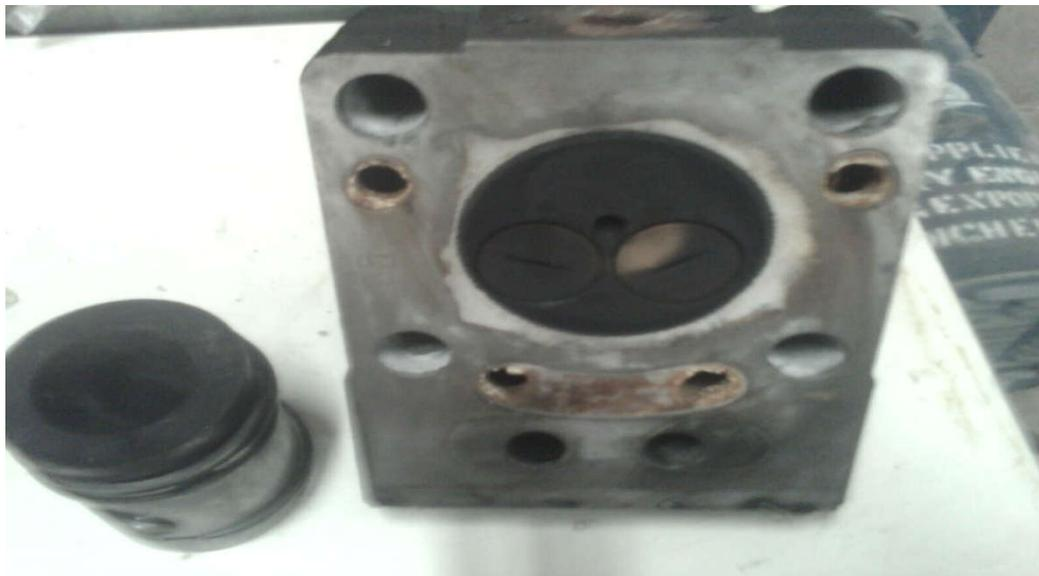
**Figure 3:** Zirconium Oxide coated piston and head
