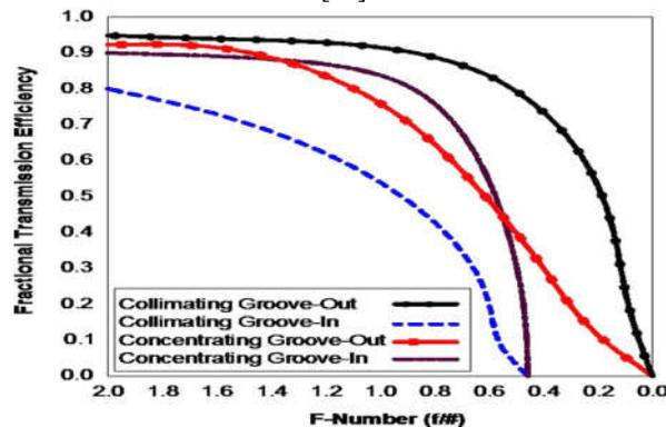
Fig.7 Transmission efficiency of lens in various mode of operation [11]
