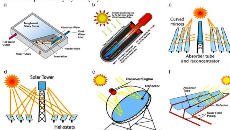
Fig.2 Types of Non-Concentrating and Concentrating collectors (a) Flat plate collector (b)Evacuated tube (c)Liner Fresnel reflector (d)Central receiver (e)parabolic dish (f)Parabolic through [11].
