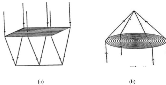
Fig.5 (a) Linear Fresnel lens (b) circular Fresnel lens
