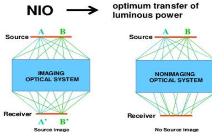
Fig.6 Imaging and non-imaging optical system [11].
