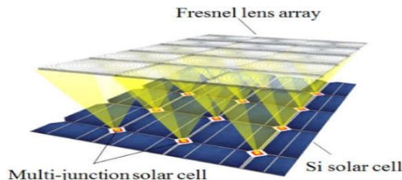
Fig.3 Concentrating sunrays on solar cell using Fresnel lens
