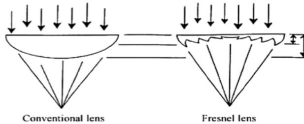
Fig.4 Difference between conventional lens and Fresnel lens
