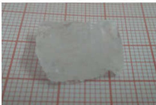
Fig. 1. A grown single crystal of urea sodium fluoride
