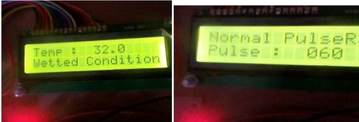
Fig. LCD displaying Infant's Urine detection condition Fig. LCD displaying Infant's Pulse Rate value
