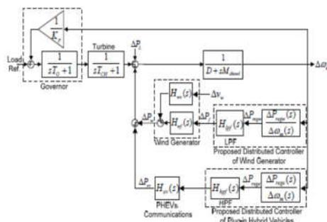
Fig.5. Block diagram representation of the microgrid frequency dynamics with a distributed cooperative controller.
