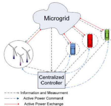
Fig. 2. Schematic view of the centralized controller.
