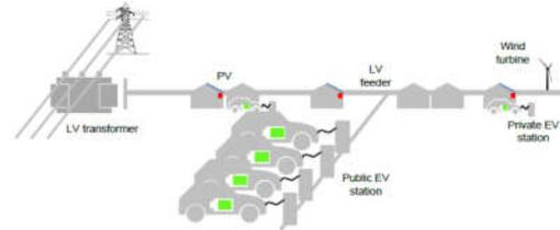
**Fig:1. EV charging infrastructures in a LV distribution grid.**
