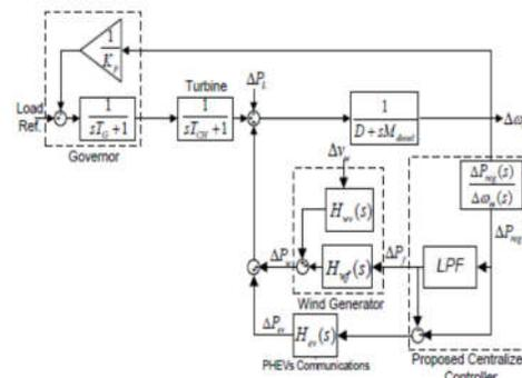
Fig. 4. Block diagram representation of the microgrid frequency dynamics with a centralized controller.
