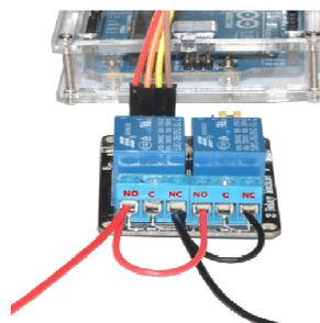
Fig. 3 Controlling Linear Actuator using Arduino
