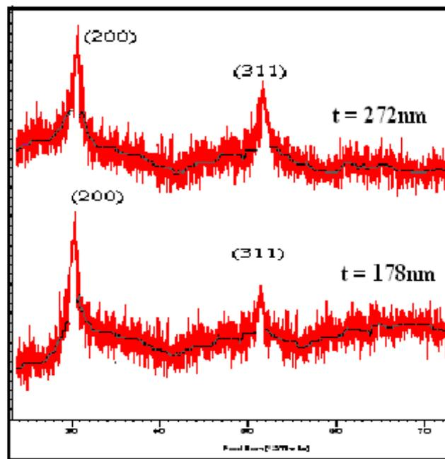
Fig. 6 XRD pattern of CdS films for thicknesses 178nm and 272nm.
