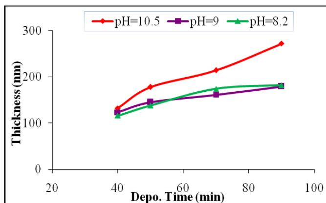
Fig.4 Variation of film thickness with the deposition time at different pH values.
