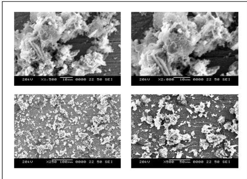
Fig. 7 SEM images of CdS films at different magnitude and thickness.
