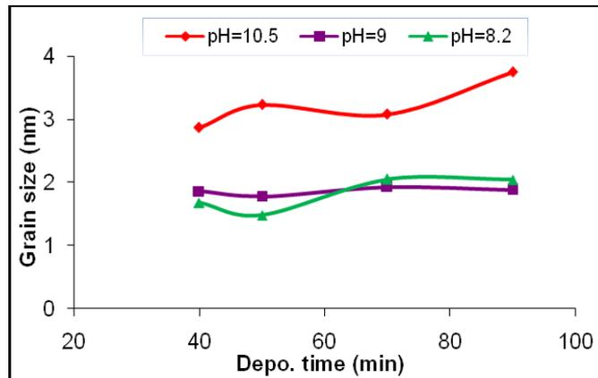
Fig. 5 shows the variation of grain size with deposition time at different pH values.
