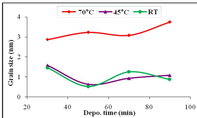
Fig. 3 shows the variation of grain size with deposition time at different temperatures.
