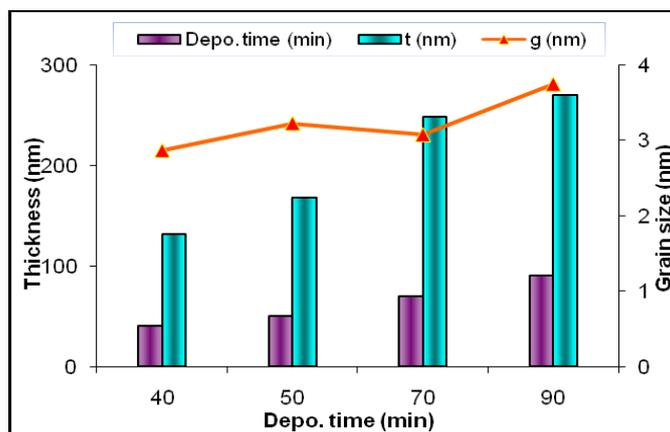
Fig. 1 Variation in film thickness & grain size with deposition time for CdS film
