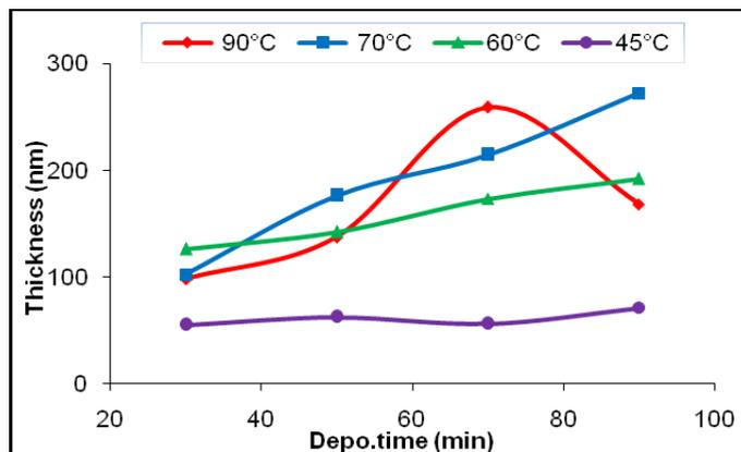
Fig. 2 Variation of film thickness with deposition time at different temperatures.
