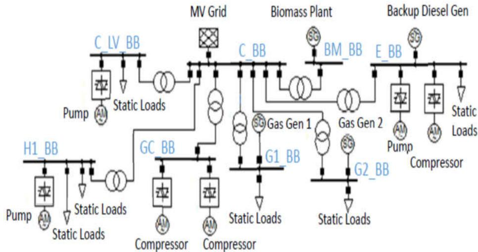
**Fig. 2.** Schematic of the modeled micro grid with 20/0.4 kV network and various DG units and load
