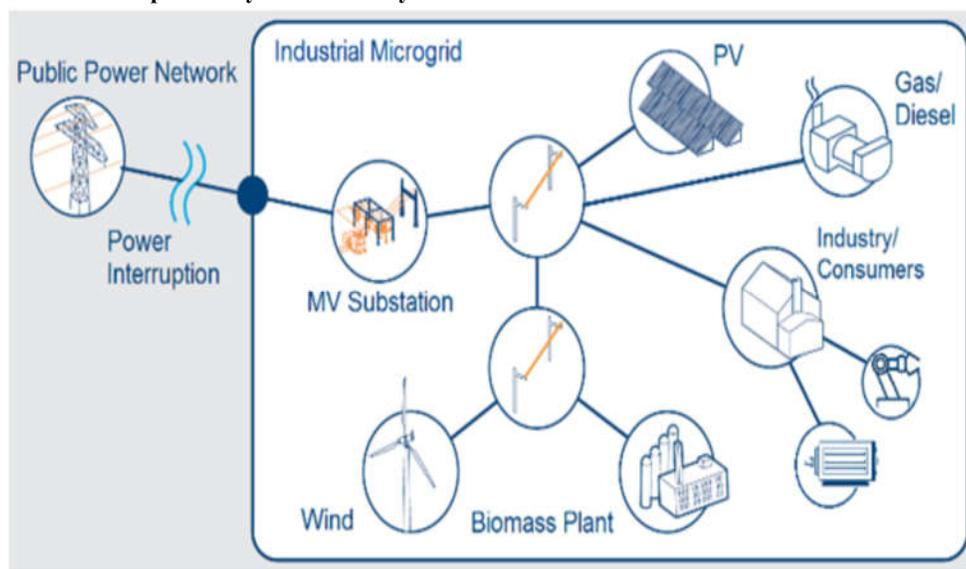
Fig: 1. A typical MG connected to the public power grid
