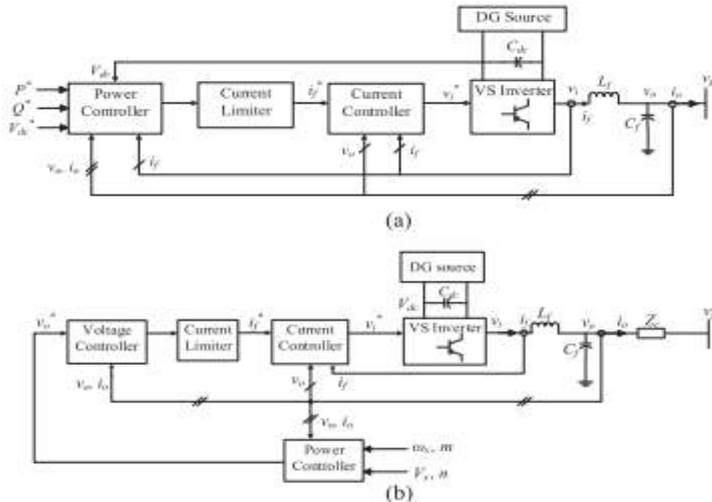
Fig. 5. Micro grid DGs control implementations. (a) Block diagram of current control scheme. (b) Block diagram of voltage control scheme.
