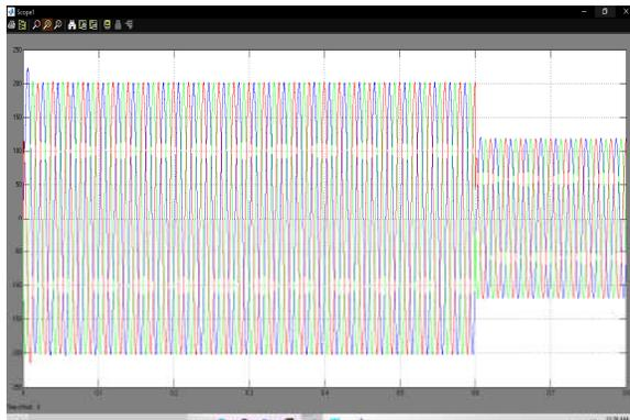
**Fig. 8.** Grid voltage (Bus 1) when current limiting is not applied to the inverters.
