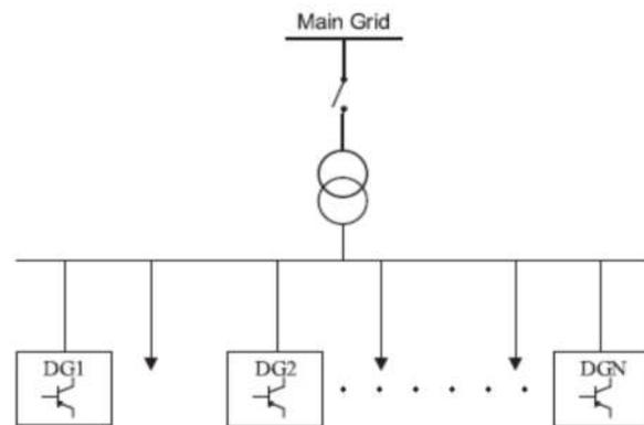
Fig: 4. Schematic diagram of a generic micro grid.
